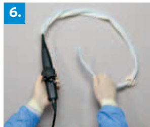
6. Fasten the cover by means of the twistlock, apply biteguard, and the probe is ready for use.
